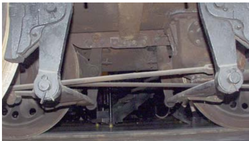
Side view between the wheel sets showing the brake rodding crossing through.
