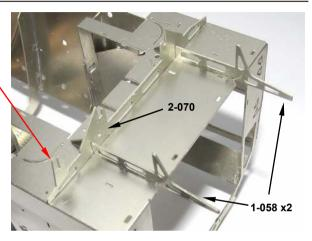
For those fortunate enough to own a Resistance Soldering Unit and using paste solders this will be easy. For the rest of us the best way is to flux liberally and feed solder to the joint where the blades project through. Move the iron tip along the surface and the solder will chase the heat source following along the underside side joint line. Keep repeating the process until complete.
