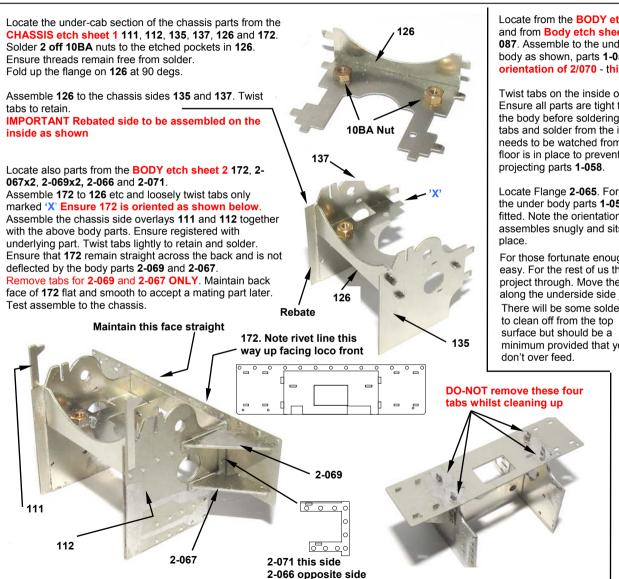
Locate from the BODY etch Part 1 1-058x2 and from Body etch sheet 2 2-070 and 2-087. Assemble to the underside of the cab body as shown, parts 1-058x2 first. Note orientation of 2/070 - this fork here -
