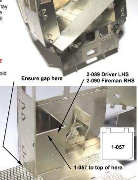
Locate the cab seat bases **2-089** and **2-090**. Fold at 90 degs and assemble to the cab interior. Twist tabs to retain. (Floor tab first, back tab and then side tab). Solder all parts. Ensure cab floor is seated to the **REAR** of the cab as far is possible leaving a gap behind the outside rear wall. Remove excess tabs and solder.
