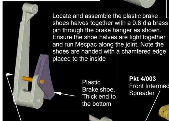
Plastic Brake shoe, Thick end to the bottom
